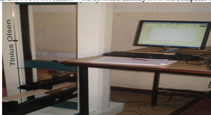
Figure 5: The Universal Testing Machine, computer and test specimen
