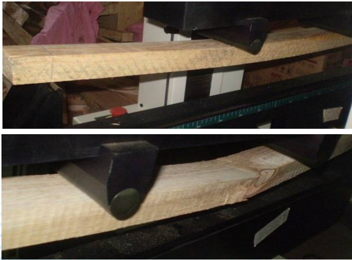
Figure 6: Structural size bending test – Pinus caribaea
